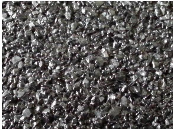
**After sealing** with our acrylic "shield": covering the granules, and filling in the spaces between them. This removes footholds for moss, encourages rapid water shedding, and keeps the granules in place.
